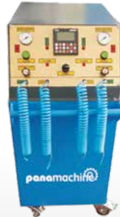
ADM OTOMATİK ARGON DOLUM MAKİNESİ AUTOMATIC ARGON FILLING MACHINE
